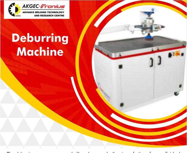
The deburring process removes built-up burrs and other imperfections from a finished surface. A burr is a ridge or area of roughness produced during the cutting of metal parts or materials. The deburring machines is equipped with a dual disc deburring motor mounted on a mechanized arm for easy manouverability. The machine table surface has a vaccum based gripping technology which helps in convenient mounting and unmounting of flat metal pieces cut by Plasma cutting machine.
